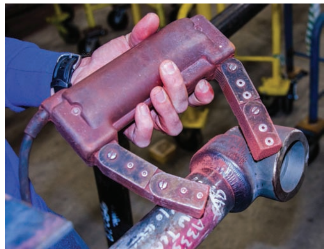
Fig. 1-8 Using a method of weld inspection known as magnetic-particle testing in pipe fabrication. This non-destructive method followed by radiograph and/or ultrasonic testing assures weld soundness for critical pipe welds. Location: Piping System's Inc. © McGraw-Hill Education/Mark A. Dierker, photographer
