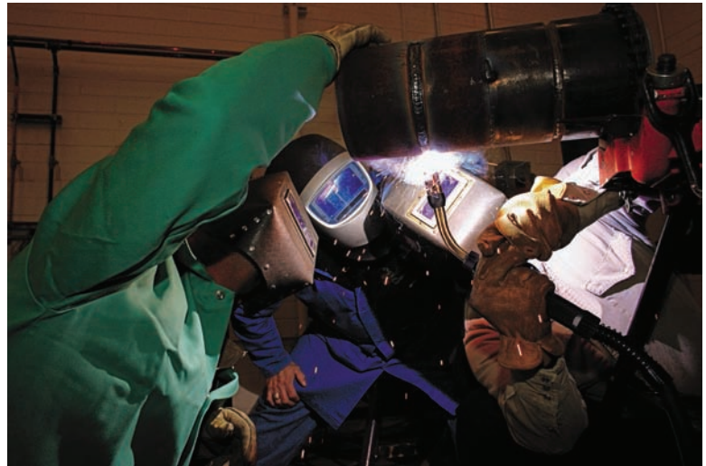
Fig. 1-7 Instructor observing students practicing for a 5G position pipe weld test. The welder is working out of the overhead position on the pipe and getting into the vertical position. The progression of the weld is uphill. The flux cored arc welding process is being used and is being applied in a semiautomatic fashion. © Miller Electric Mfg. Co.
